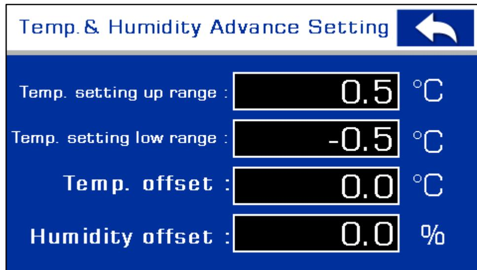
**Temp. setting up/low range:** "default:  $\pm 0.5^{\circ}\text{C}$  " Set Temp. control range in the ECO-IR setting screen.
